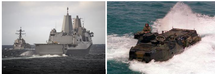
San Antonio-class Flight II landing dock ships (left) and the Marine Corps Amphibious Assault Vehicle (right).
