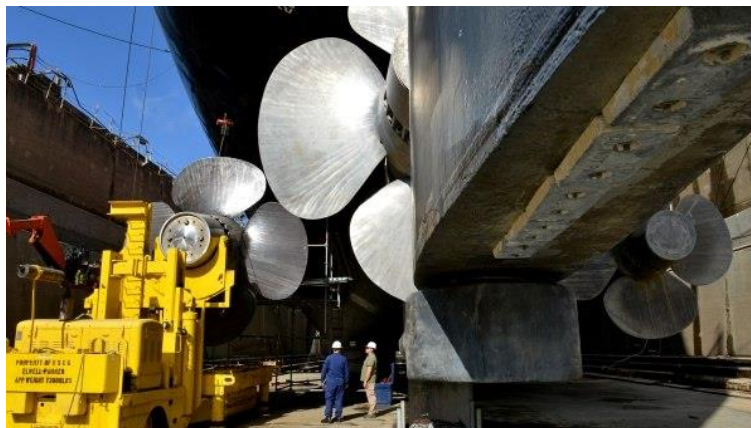
A contractor and a Polar Star crew member assess progress being made reassembling the cutter's port side hub while the cutter underwent extensive repairs at a dry dock facility in Vallejo, Calif., on Oct. 3, 2018.
